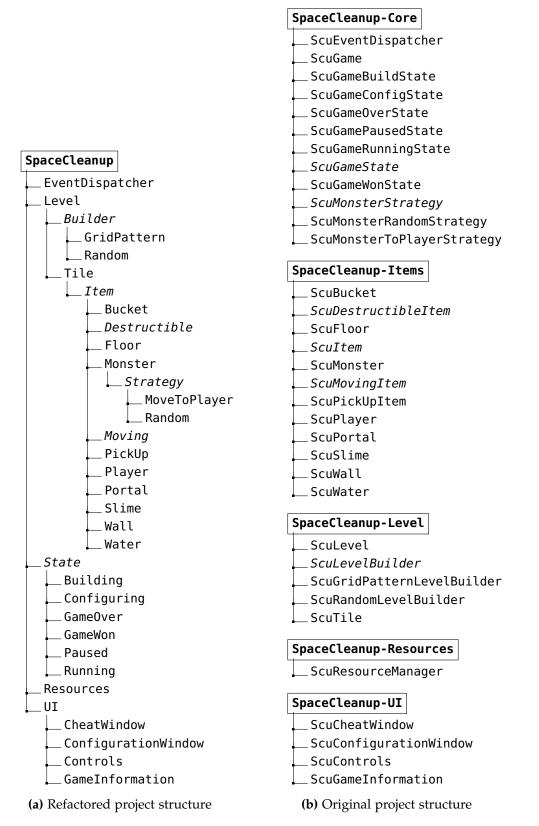
**Figure 5.7.:** Example: Hierarchical decomposition. SpaceCleanup game implementation with/without hierarchical decomposition.
