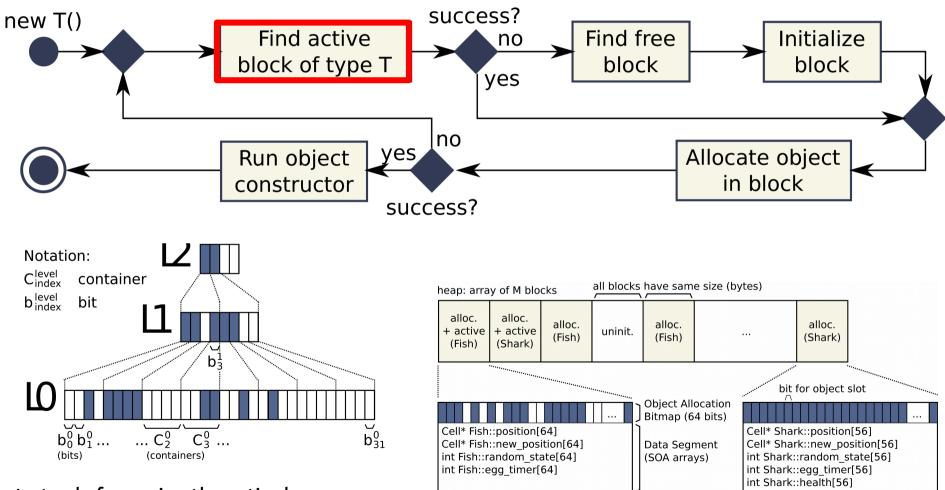
Instead of scanning the entire heap: Traverse a hierarchical bitmap
